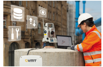
Deformation monitoring system
