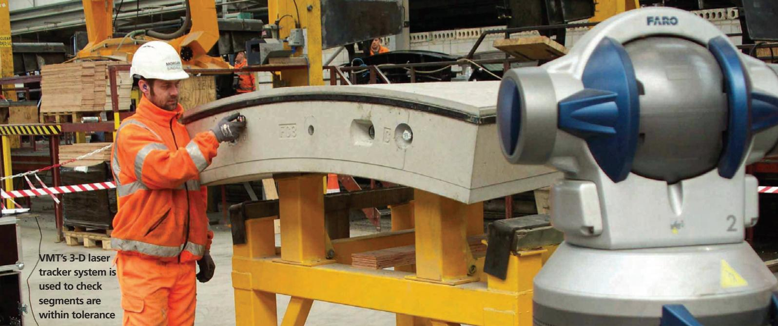
VMT's 3-D laser tracker system is used to check segments are within tolerance
