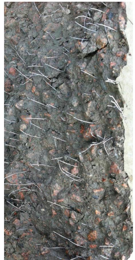
**Lee's segments employ 30kg/m<sup>3</sup> of Dramix steel fibre reinforcement**
