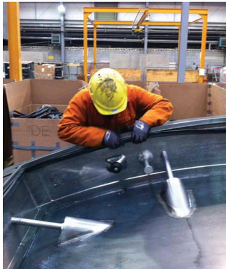
**Above: PDT's gaskets are a push fit into the gasket recess of the CBE moulds**
