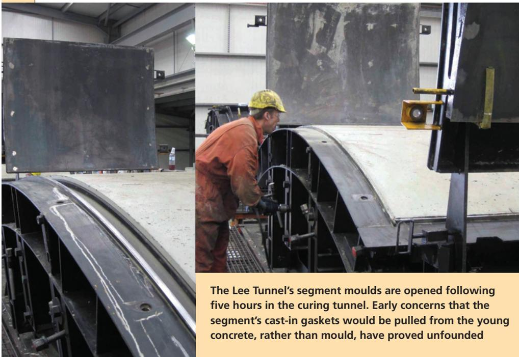
**The Lee Tunnel's segment moulds are opened following five hours in the curing tunnel. Early concerns that the segment's cast-in gaskets would be pulled from the young concrete, rather than mould, have proved unfounded**
