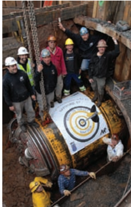
Above: 2010 - First microtunnelling curve drive in the US successfully completed with a radius of 414m and precisely guided by a VMT navigation system.
